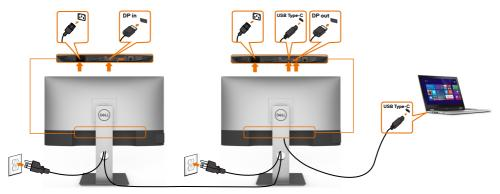
**NOTE:** The maximum number of supported U2721DE via MST is subjected to the bandwith of the USB-C source. Please refer to "product specific problems –No image when using USB-C MST".
