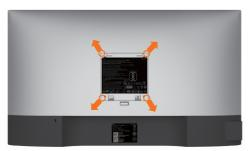
MOTE: Use M4 x 10 mm screws to connect the monitor to the wall-mounting kit.
