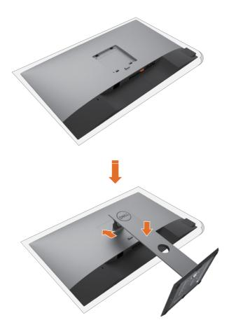
**1** Remove the monitor protective cover and place the monitor with its front facing downward on it.
